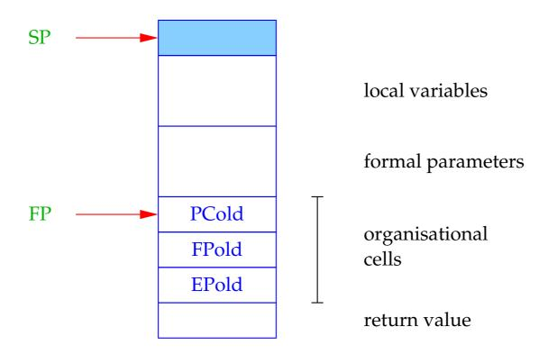
$FP \cong Frame Pointer$ ; points to the last organizational cell and is used to address the formal parameters and the local variables.
