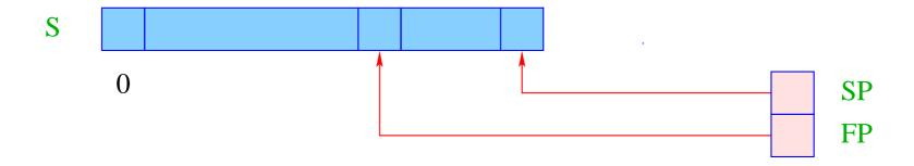
S = Runtime-Stack – each cell can hold a basic value or an address;
