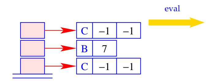
0 alloc 2 3 rewrite 2 3 mkbasic 2 pushloc 1 2 pushloc 0 2 loadc 7 3 rewrite 1 3 eval 3 slide 2
