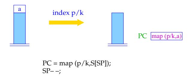
The function map() returns, for a given predicate and node content, the start address of the appropriate try chain :-)
