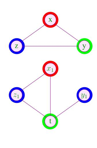
Interference graphs for minimal live ranges on basic blocks are known as interval graphs:
