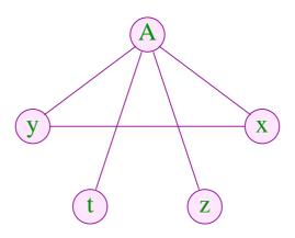
Variables which are not connected with an edge can be assigned to the same register :-)
