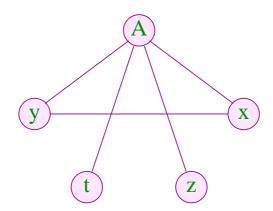
Variables which are not connected with an edge can be assigned to the same register :-)
